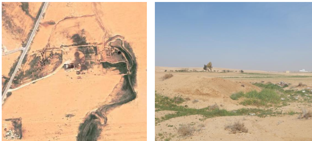
Figure 17. The three earth dams on satellite imagery (left), and the eroded wings of the most upstream embankment (right).
