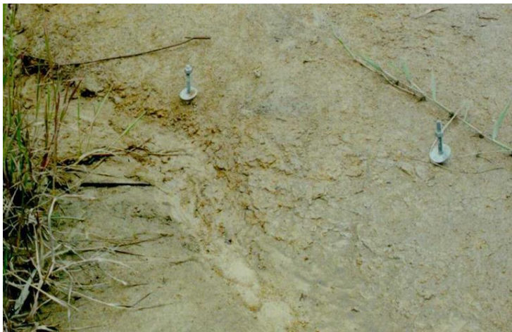
Figure 21. Example of erosion pins with washers (source: SERC Carleton College).
