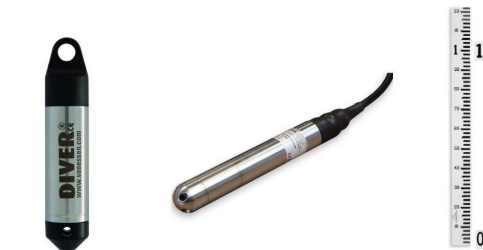
Figure 20. Examples of pressure sensors. The left sensor represents an absolute pressure and temperature sensor with the datalogger integrated in the housing. The right sensor is air pressure compensated with a capillary vent in the cable.
