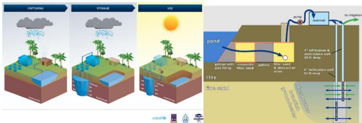
Figure 24: Example of a small-scale MAR system implemented by Acacia Water in Bangladesh (source: Acacia Water, 2015)
