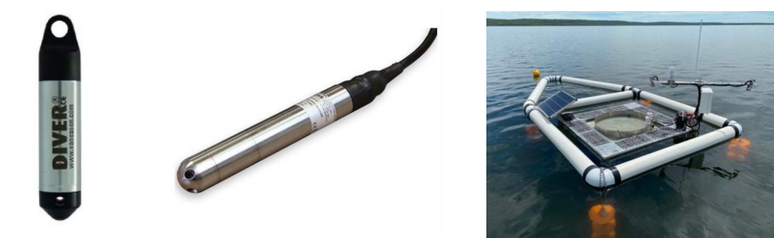
Figure 19. Example of pressure sensors (left and middle). The left sensor represents an absolute pressure and temperature sensor with the datalogger integrated in the housing. The middle sensor is air pressure compensated with a capillary vent in the cable. On the right an example of a floating evaporation pan is shown.
