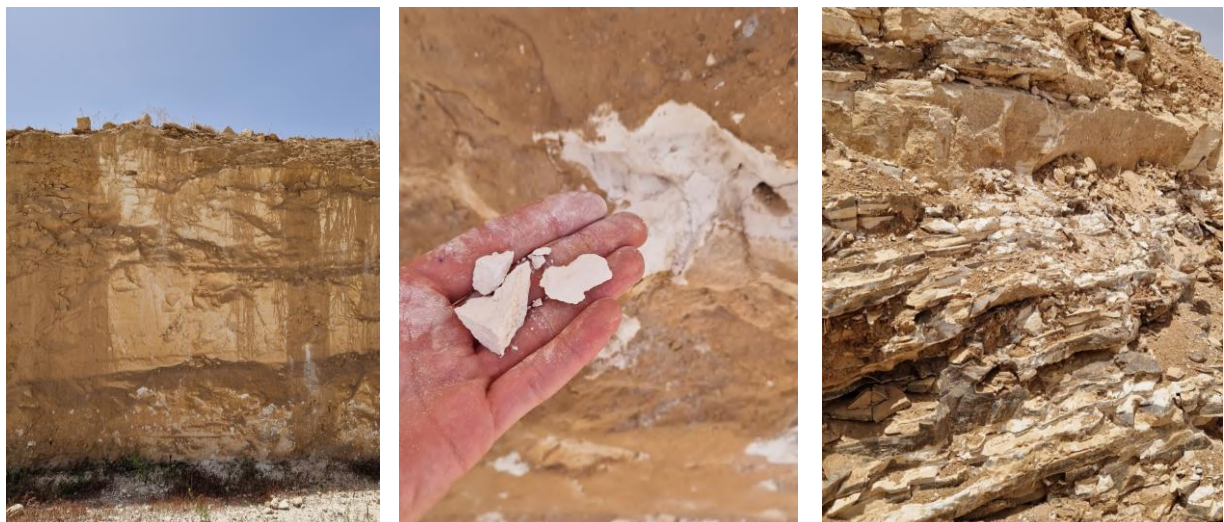
Figure 4. Chalk Marl from the Muwaqqar formation (left and middle) and the limestone-chert from the B4/B5 formation (right).
